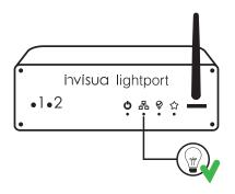
Verify that the second LED is ON to confirm internet connection. (Blinking indicates having an IP address obtained, full ON indicates internet connection)
