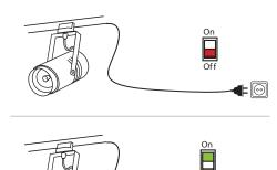
Within 30 sec. after pressing button #1, turn the Masterspot 2 Track fixtures OFF and ON again, by disconnecting and reconnecting the 230V power.
