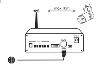
Connect the Invisua Lightport to your local network router (with internet access) via the supplied LAN cable. (Recommended maximum distance Lightport-fixtures: 10m. line of sight)
