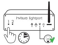
Press button #1 on the Lightport for 5 sec. to initiate commissioning of your system. (lamp indicator LED on the Lightport will turn ON)
