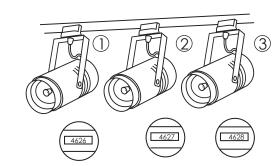
It is recommended to position the fixtures ordered by serial number. In that way the fixture sequence in Invisua Create will be identical.
