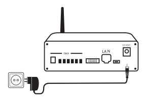
Power the Invisua Lightport via the supplied 12V power supply.
